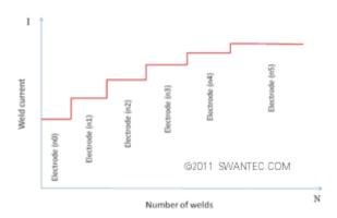
**Electrode tip-dressing** is a method to mechanically re-shape or abrasively clean the electrode tip after a certain number of welds to preserve nearly the same initial tip diameter and surface conditions. In this way, the welding process can be controlled at the same process parameters or slightly regulated by an adaptive control system to maintain consistent weld quality.
