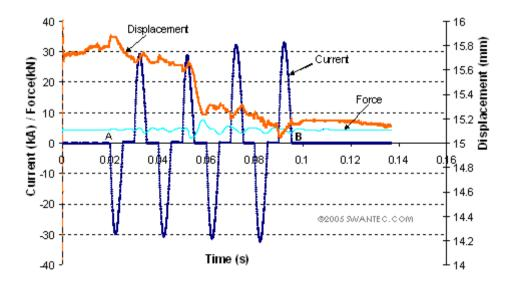
Electrode degradation and tip dressing
